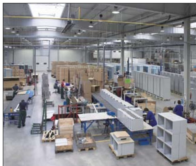
Assembly of data communication cabinets
