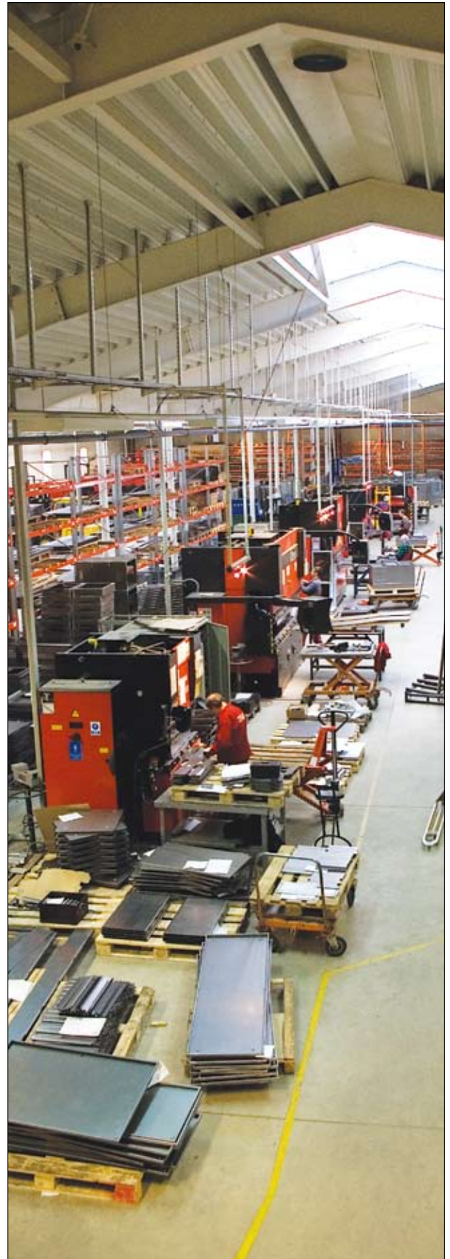
Hall housing bending brakes
