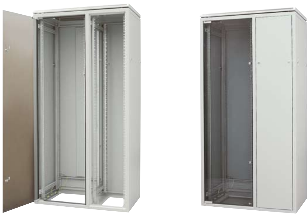
SZB cabinet 1000 mm wide, double-sectioned. Left section equipped with 19" mounting profiles. Right section with mounting angles in 300 mm spacing. Tailor made.
