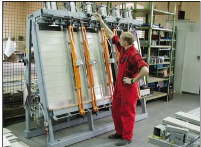
Fastening of aluminium panels for outdoor cabinets shields
