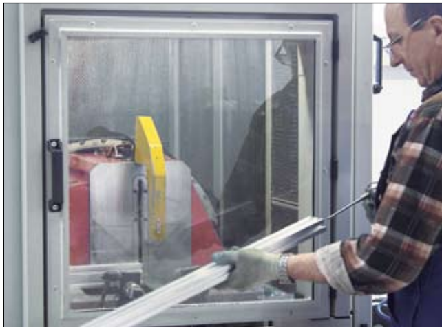
Cutting of aluminium profiles used in frames of outdoor cabinets
