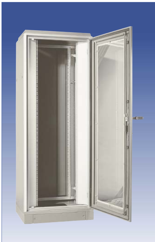
SZA cabinet 800 mm wide, front door with glass and 3-point rod-latch lock
