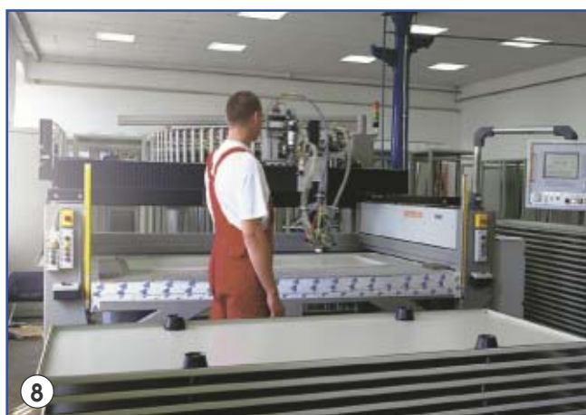
photo 6: automated powder paint shop, photo 7: numerically controlled punching machinery, photo 8-9: robotic sealant machinery.
