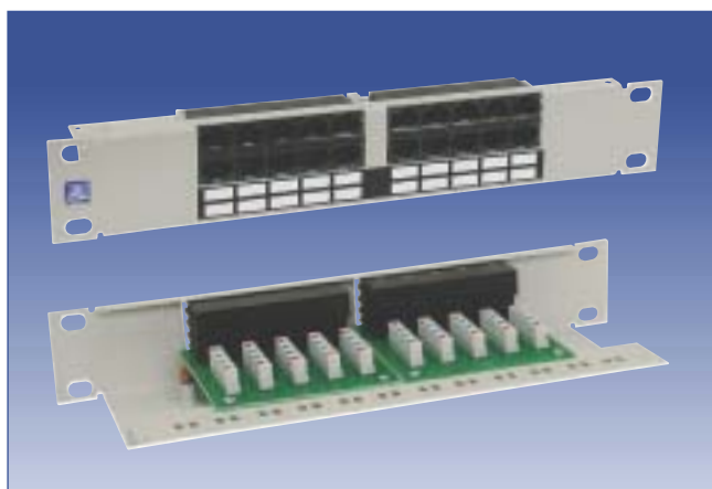
Telephone patch panel UTP 10" x 1U, cat. 3, 20 ports - cat. no. 891-220 Weight: 0.3 kg Dimensions (width x height x depth): 275 x 44 x 55 mm Electrical parameters as in panel 807-155 (page 29)
