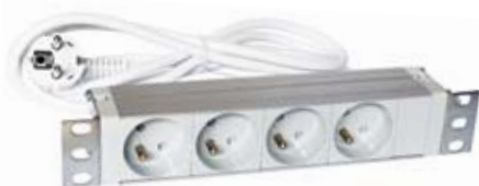
Power strip 10" x 1 U, 4 sockets type E (CEE 7/5), voltage rating 230 V AC, maximum current 10 A, cable 1.8 m with universal plug, body made of anodized aluminium - cat. no. T-SO-891-317
