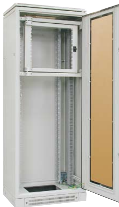
SZB cabinet 42 U height, 800 mm wide with 10 U swing frame. Non-standard version (detailed description of swing frames SZB cabinet with easy adjustment of 19" mounting profiles - see page 88).
